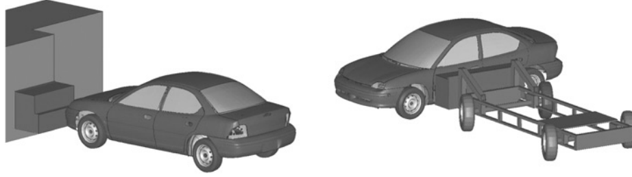
Fig. 8 Finite element models for offset-frontal and side impacts.
